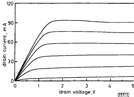
Fig. 2 Typical DC current-voltage characteristics of high-low doped GaAs power MESFET with gate width of 300  $\mu\text{m}$
