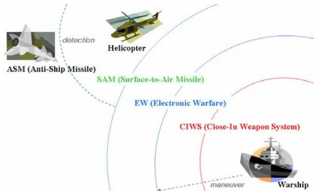
Figure 3 Defense of a Naval Ship Against Anti-Ship Missiles
