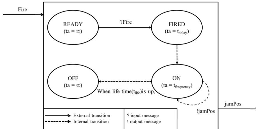
**Fig. 2.** Design of the jammer model ( $t_{\text{delay}}$  is the time of the firing delay.  $t_{\text{frequency}}$  is the interval time required to send output messages.  $t_{\text{life}}$  is the total lifetime of the jammer).
